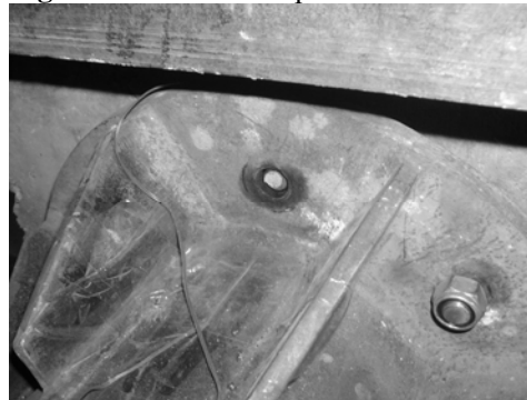
Fig. 17: Bolt Fracture in Stiffened Specimen
